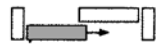
Scheme A* Moving sashes 1 Max. width (mm) 6,700 * Left hand shown above, right hand also available
